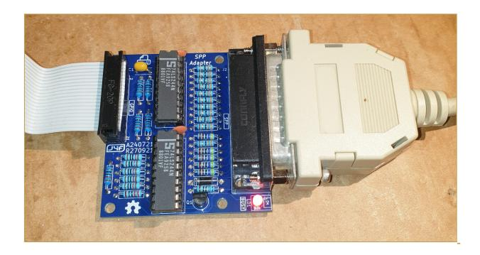
The cable to use for the printer is the common *parallel printer cable*, with a DB-25 connector at one side and a Centronics connector at the other:
