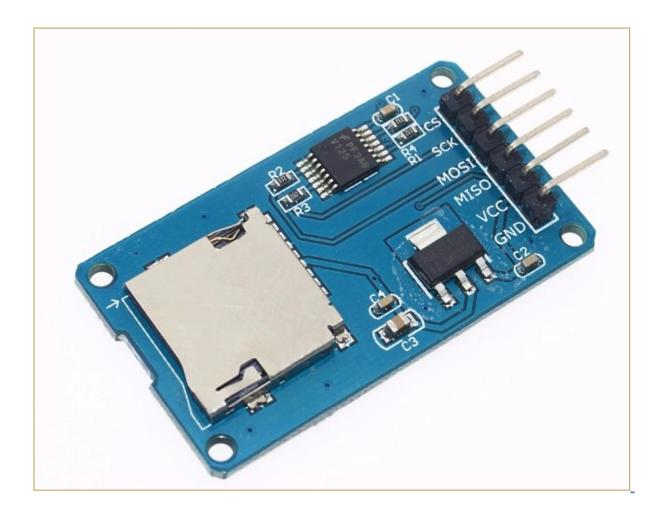
Pay attention on how and where you plug the module in (the only right connector for it is **J6** marked as **SD-MOD**). If you plug it in the wrong connector or in the wrong way it is possible cause permanent damages to both the module and the Z80-MBC2 board!
