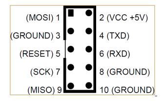
In the previous picture it is possible see that pins 4 (TXD) and 6 (RXD) are not at GND as expected by the standard ICSP port, and pin 3 is not NC.
